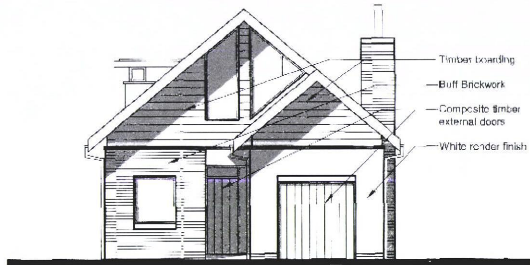
NORTH EAST ELEVATION (TO EGLANTINE WALK)
