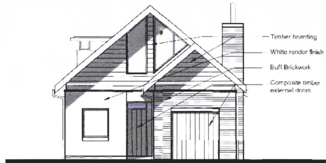
NORTH EAST ELEVATION (TO EGLANTINE WALK)
