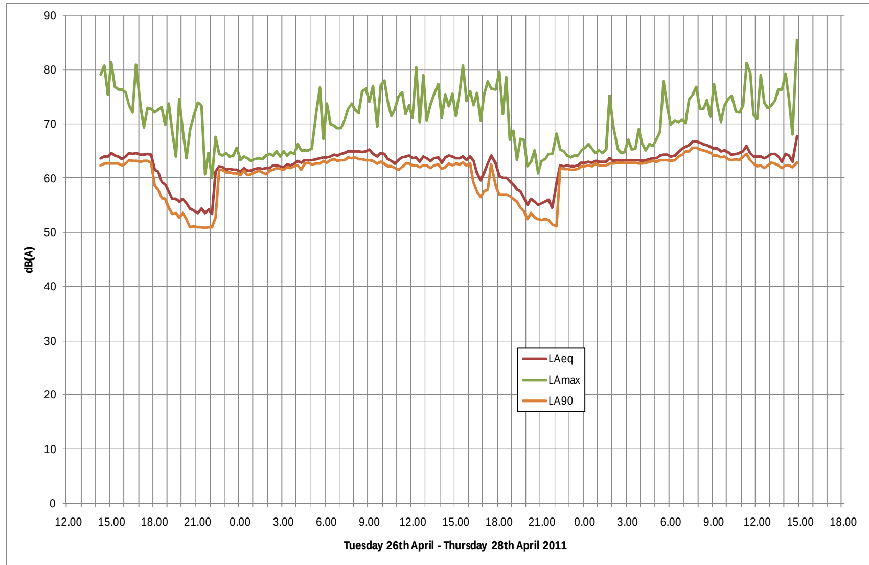
FIGURE 2 - MEASURED NOISE LEVELS, LANGSTONE TECHNOLOGY PARK
