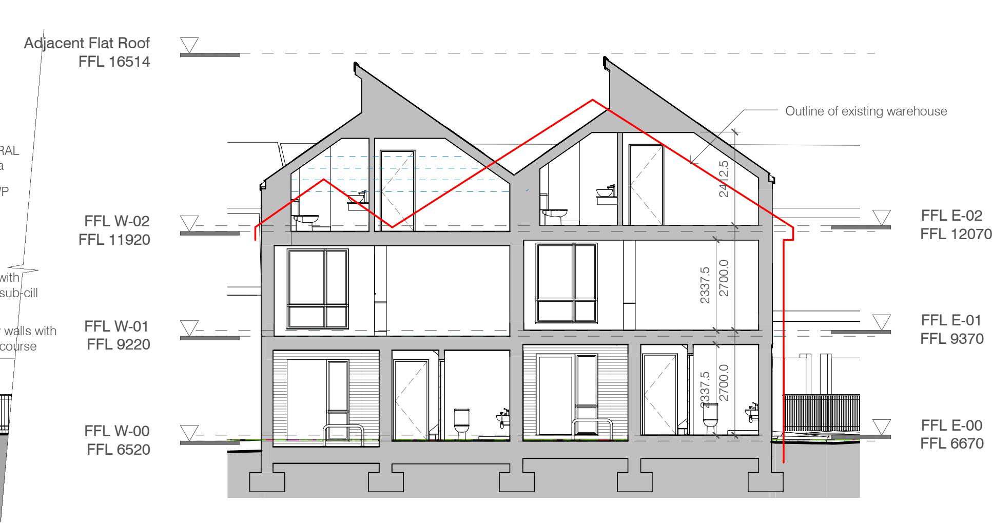
5. Proposed Section A-A scale 1 : 100
