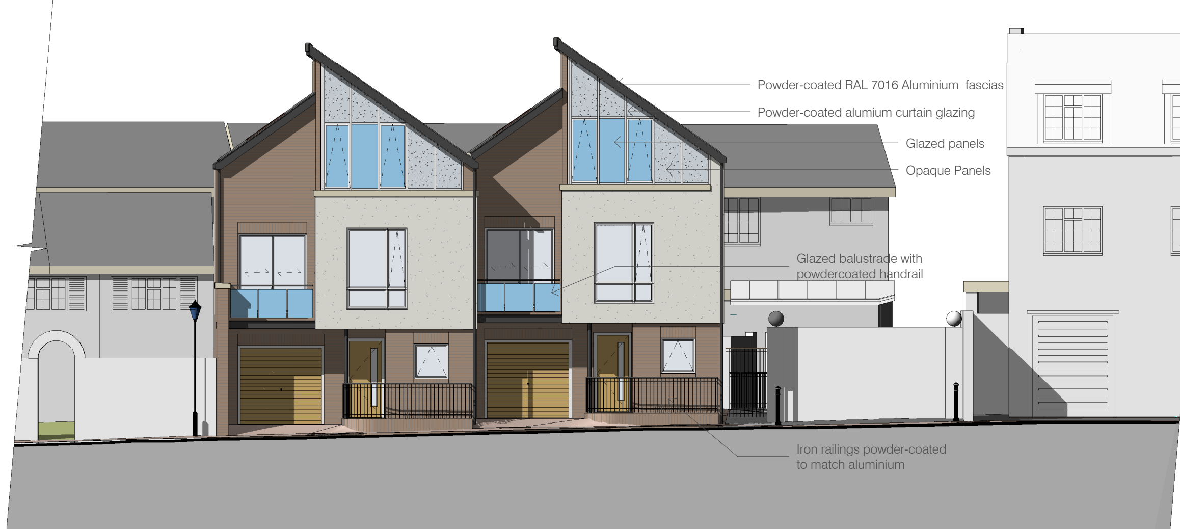
9. Proposed South Elevation scale 1 : 100
