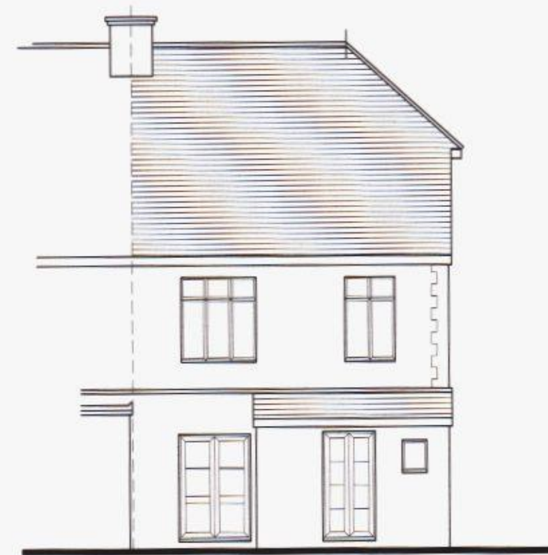
EXISTING REAR ELEVATION 1/100.
