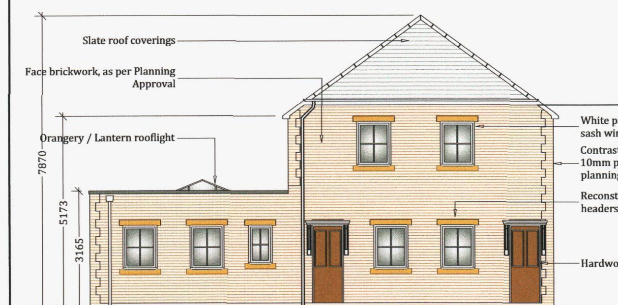
UNITS 3, 4 & 5 - FRONT (WEST) ELEVATION 1:100
