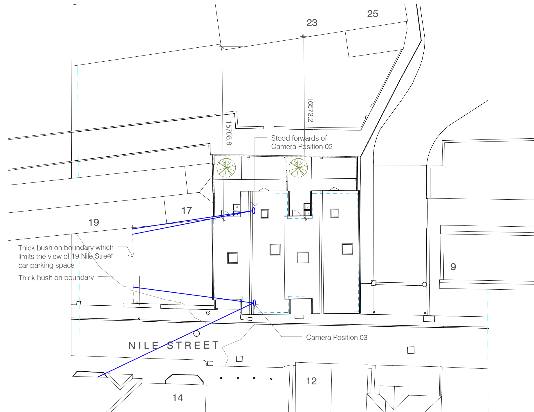
2. Proposed Site Layout Sight Lines scale 1 : 200
