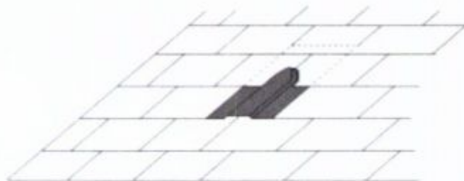
Fig 9. Batstones can be fitted in the middle of a slate roof but more lead and considerably more labour is involved.
