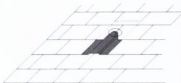
Fig 10. To allow bats into the loft, a hole may be cut in the roofing felt. The hole needs to be cut adjacent a rafter or wall to enable the bats to crawl in and out.
