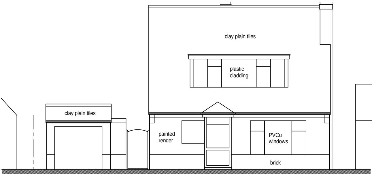
Existing East Elevation
