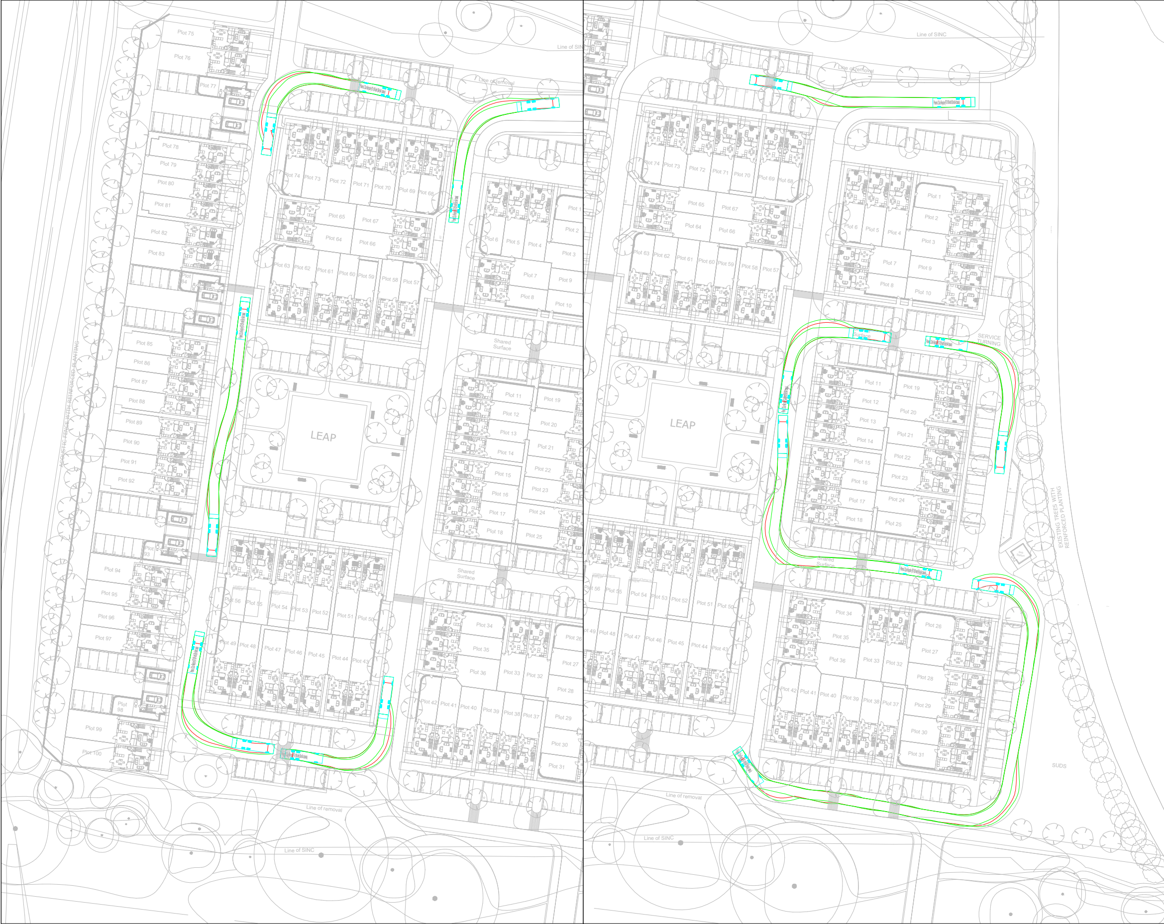
WESTERN SIDE OF SITE - REFUSE TRACKING
