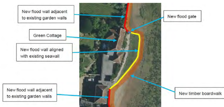
Figure 4.14: Sketch plan of the outline design seawall and boardwalk alignment at Green Cottage
