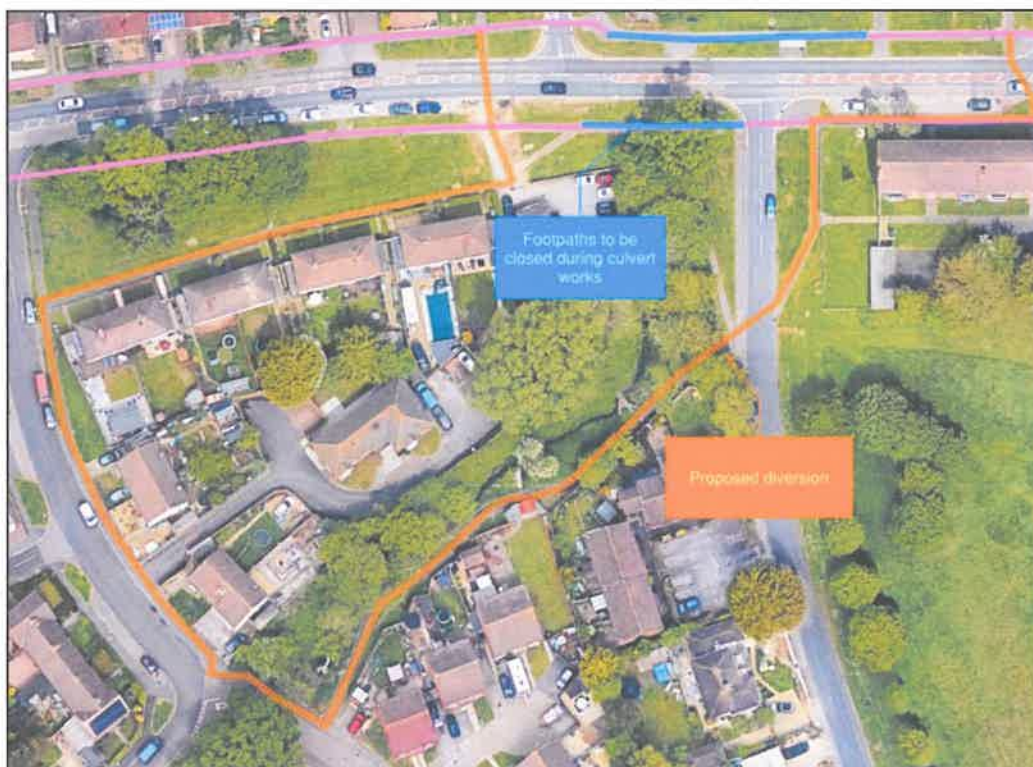
Figure 13-3 –Riders Lane PRow Closure and Diversion
