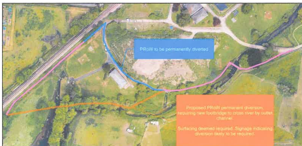
Figure 5-3 – Meyrick Road PRow Closure and Diversion
