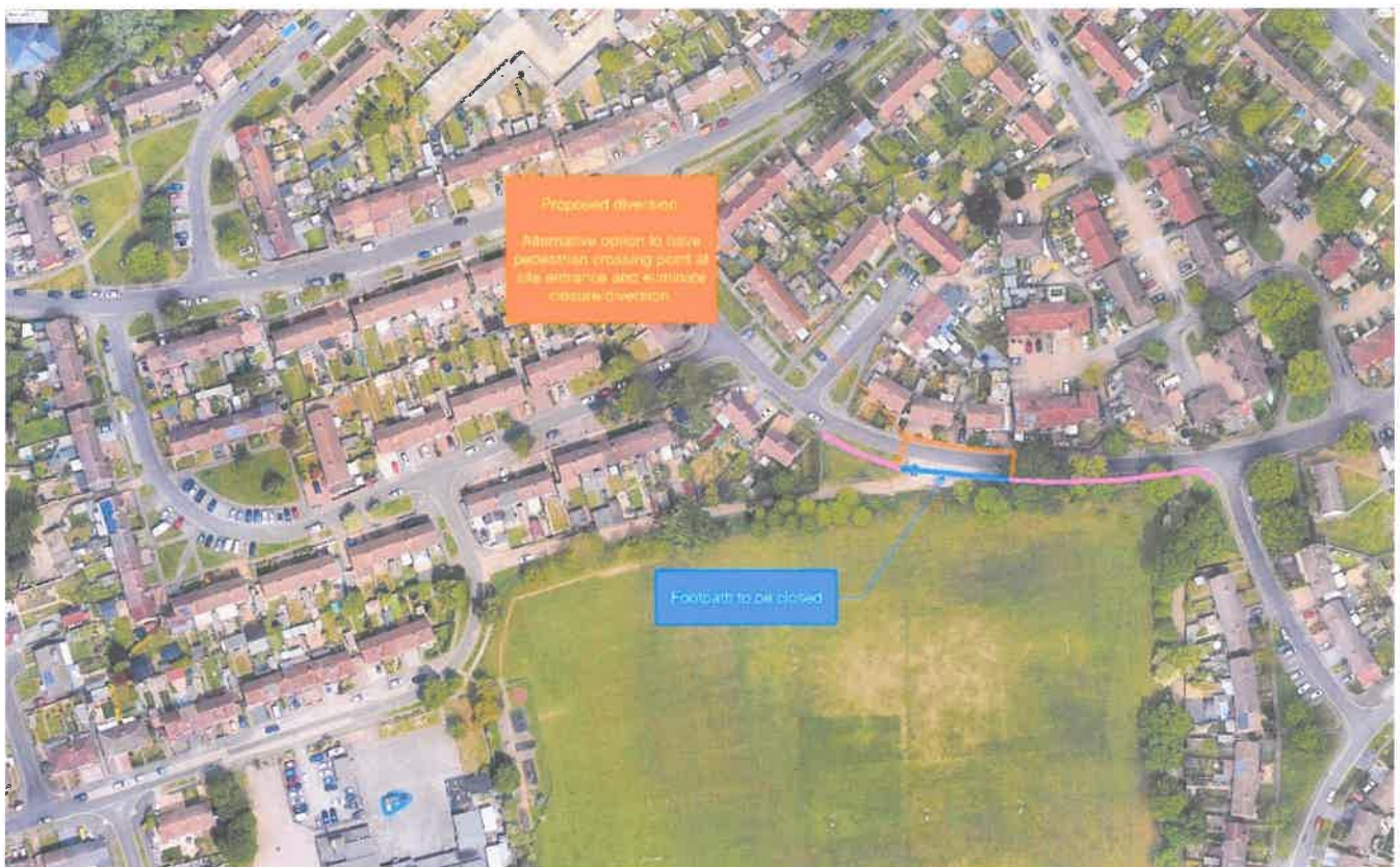
Figure 6-4 – Hooks Farm Way Footpath Diversion
