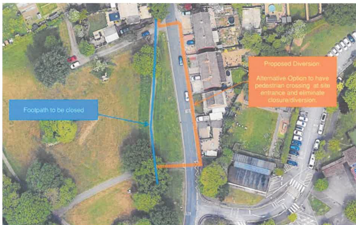
Figure 7-4 – Stockheath Lane footpath diversion
