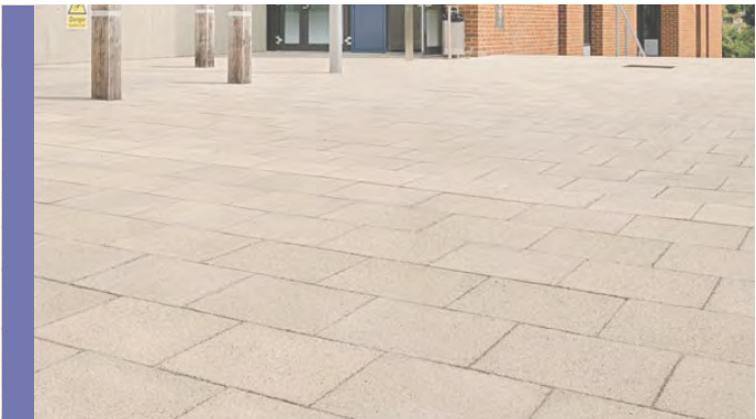
450mm x 450mm x 35mm deep PC concrete Saxon Natural coloured, textured finish slab paving by Marshalls or similar approved
