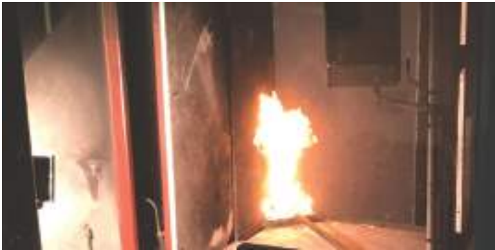
■ Photograph of EN 13823 (SBI) Testing
