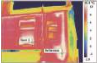
Thermal image of rear elevation and gable before refurbishment shows excessive heat loss through walls, windows and waste pipe penetrations
