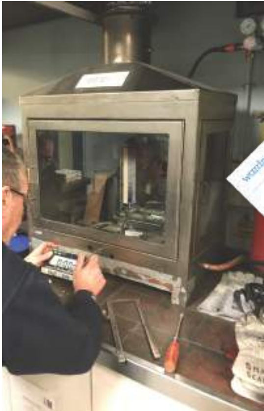
■ Photograph of EN ISO 11925-2 Testing
