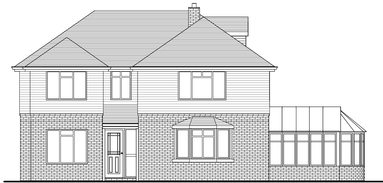
Existing West Elevation 1 : 100
