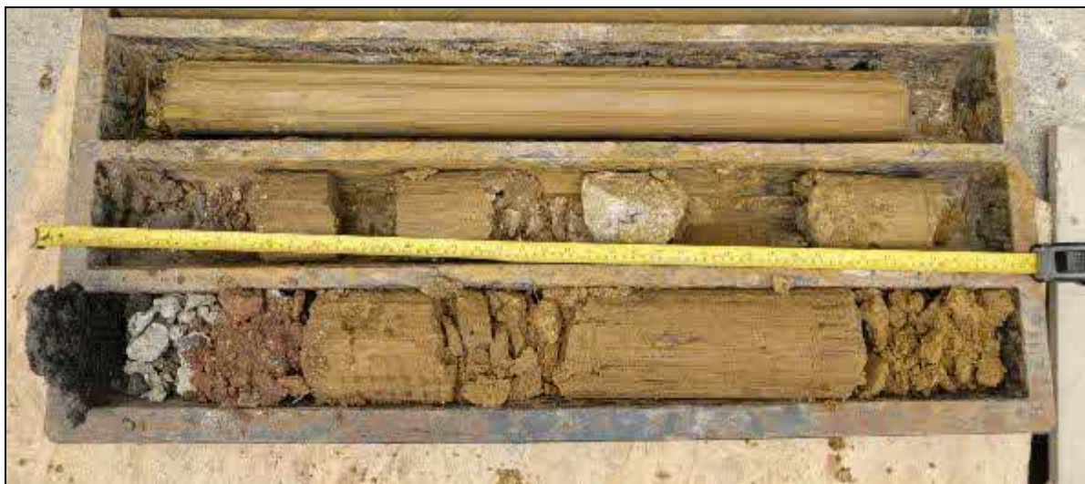
Photograph 3 Removed soil material - Location BH.03
