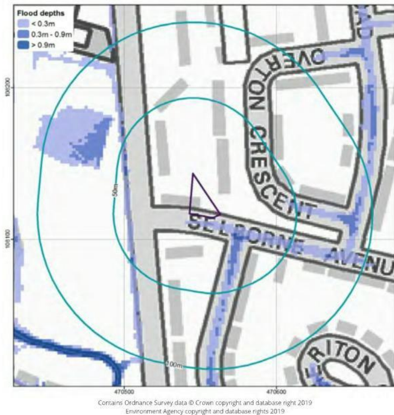
Figure 5 EA 1 in 100 year surface water pluvial flood event
