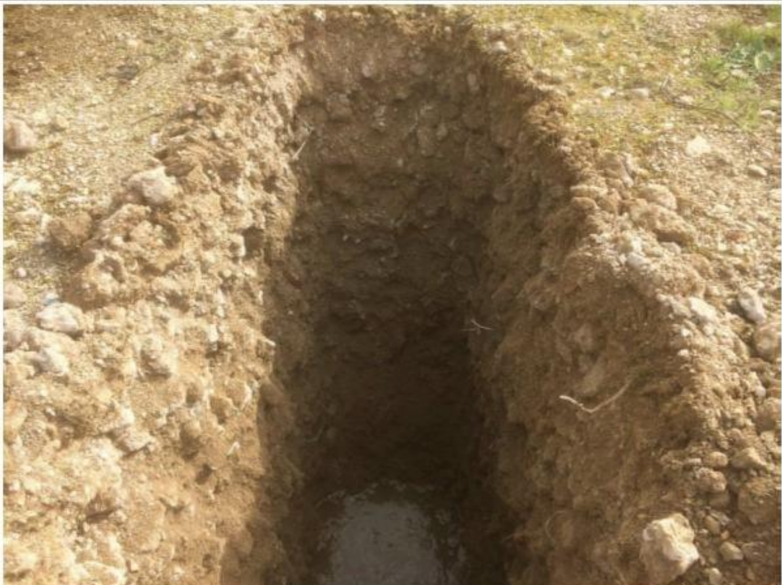
PLATE 10 – TP3 made ground to full depth to groundwater at 2.3m
