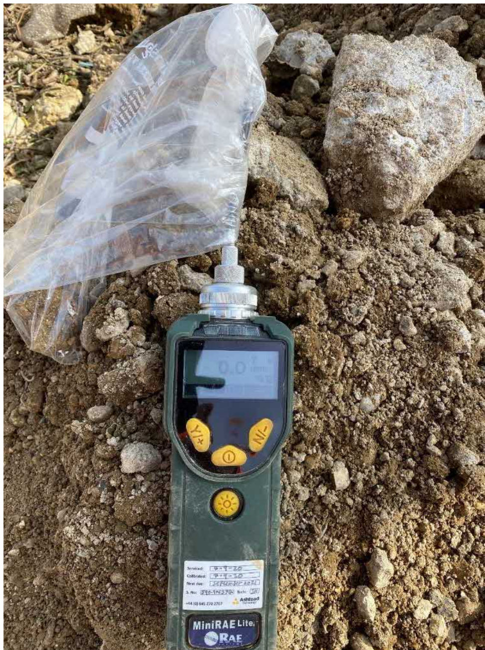
Figure 11 – Trial Pit Delineation PID Headspace Analysis (ESL102)
