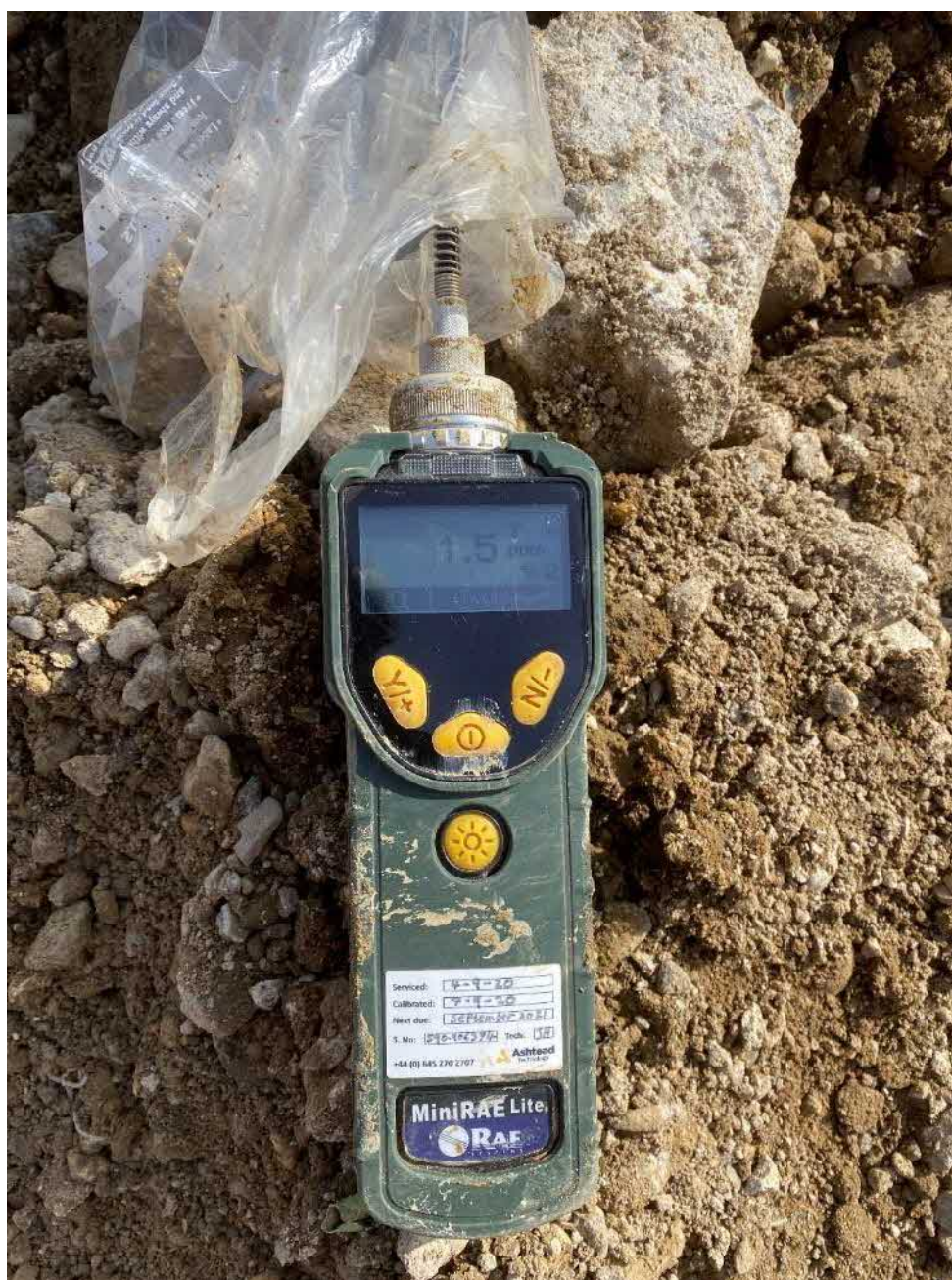
Figure 10 – Trial Pit Delineation PID Headspace Analysis (ESL109)
