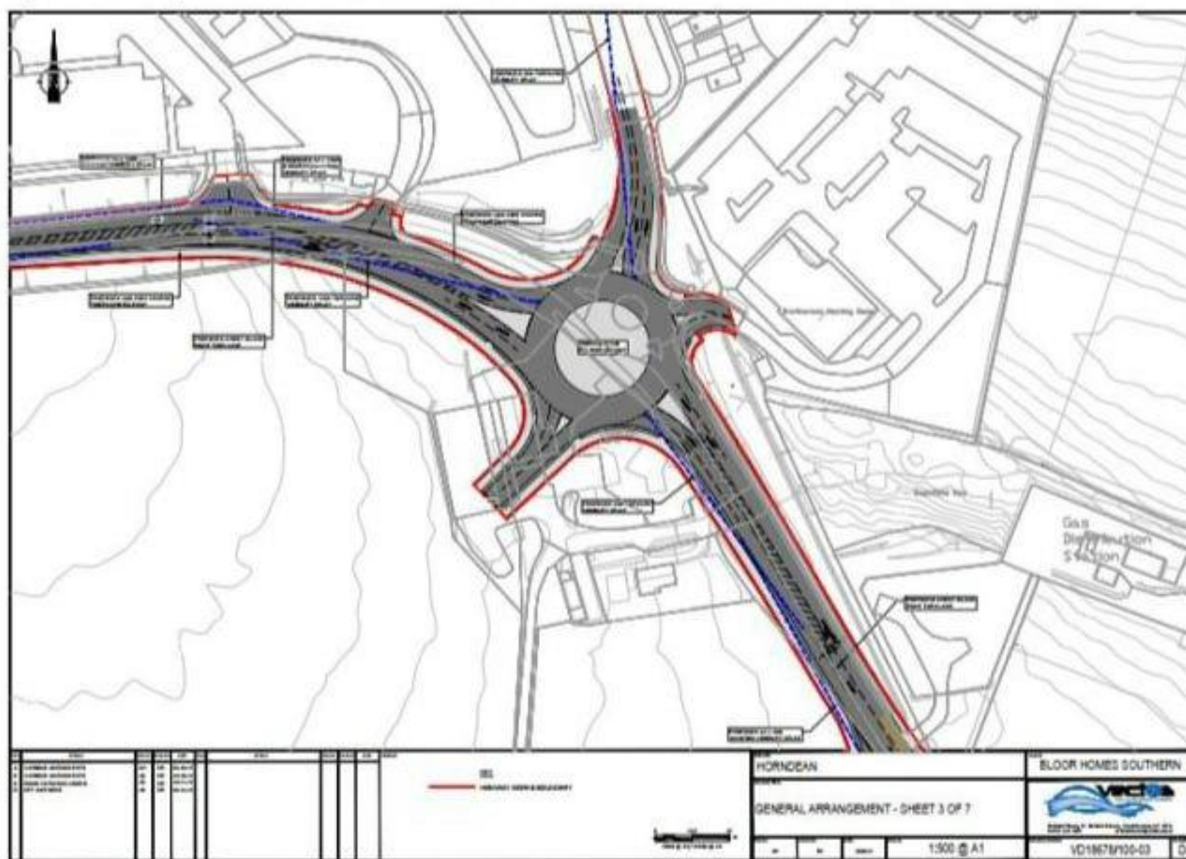
Figure 5-5 - Improvements to the Dell Piece East/B2419 Roundabout
