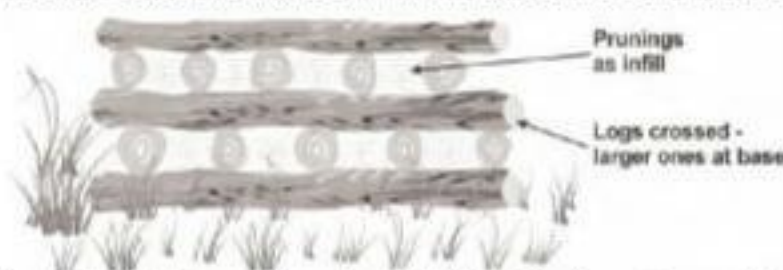
Figure 1.1 Schematic of a wildlife pile (courtesy of Steve Wilson and Robert Bray of Sustainable Drainage Associates)
