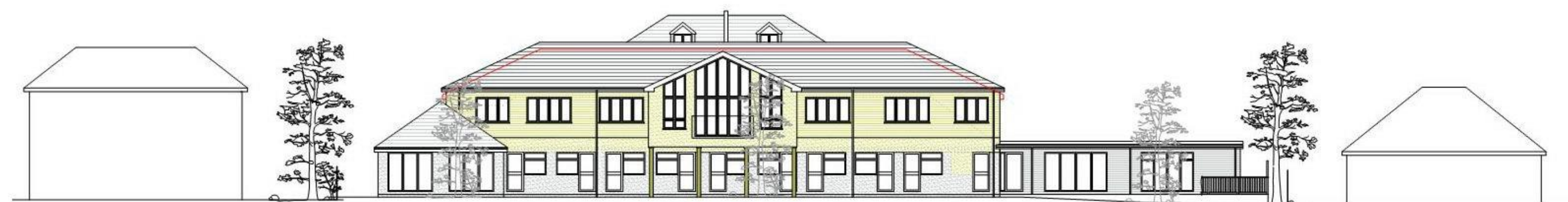
Proposed West Elevation - 1:200 - Showing Neighbouring Properties
