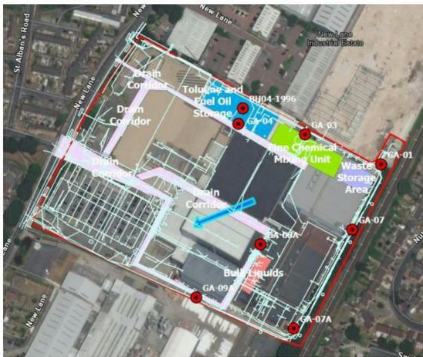
Figure 3 - Site Plan showing the location of potentially contaminating land uses (blue arrow signifies interpreted groundwater flow direction)
