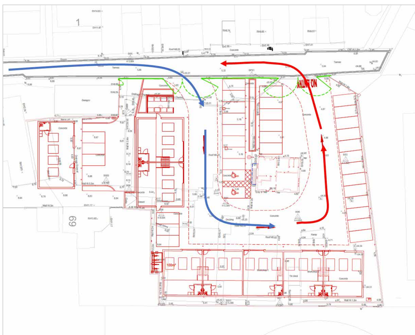
Figure 4.4: HGV Access Arrangements
