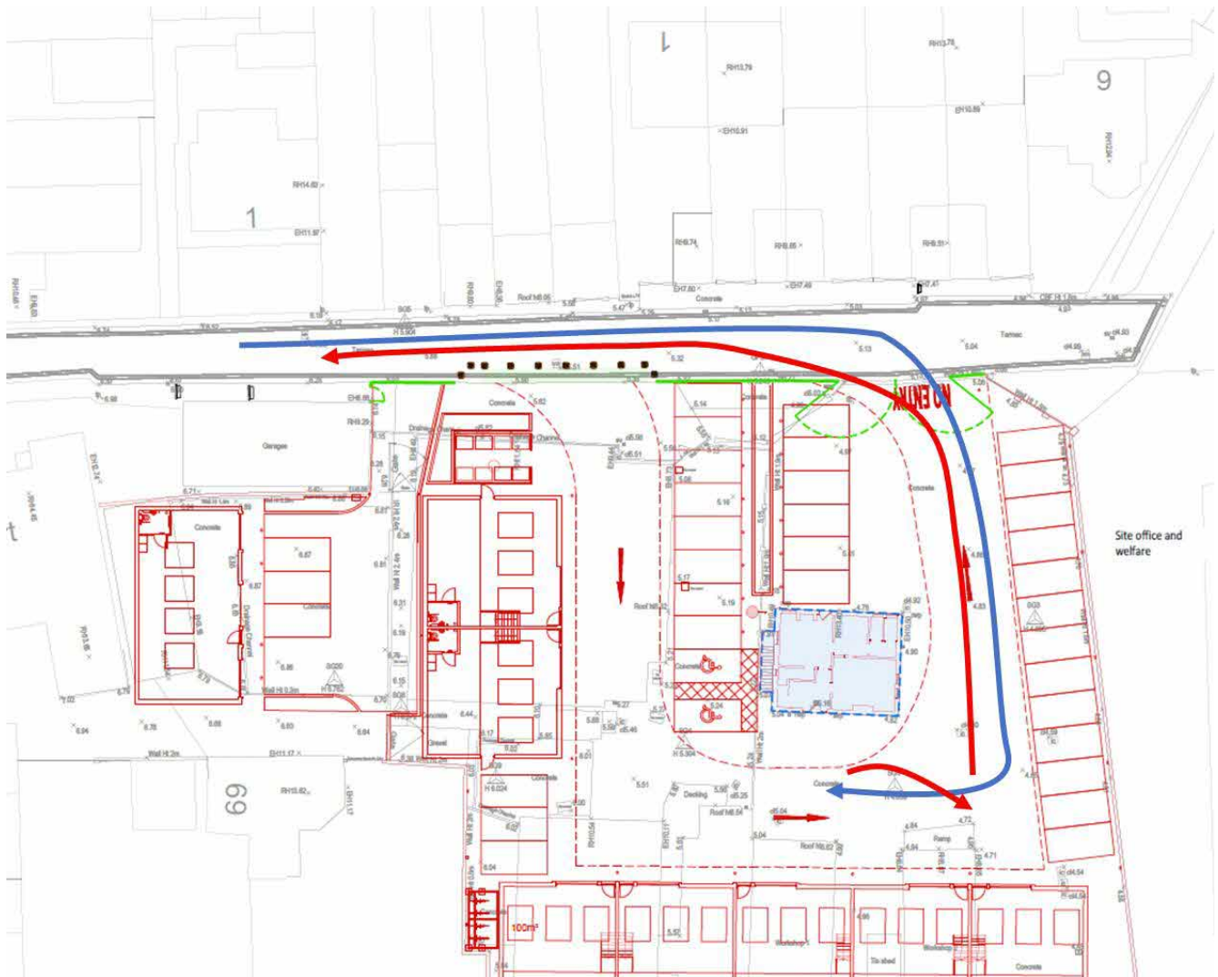
Figure 4.3: Phase 3 Give / Take Arrangement (Access Construction)
