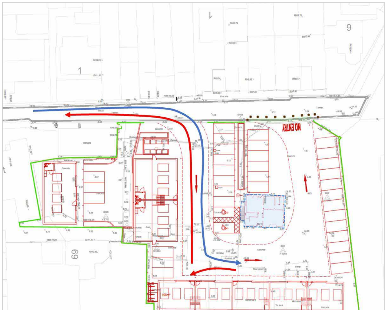
Figure 4.4: Phase 3 Give / Take Arrangement (Egress Construction)
