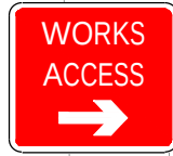
Works Access sign as per Traffic Signs Manual Diagram 7301
