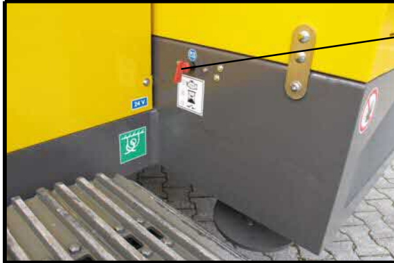
Battery main switch
