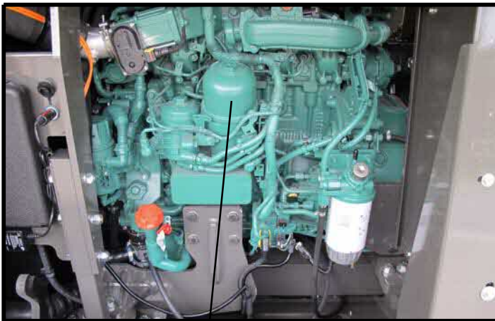
Engine oil filter
