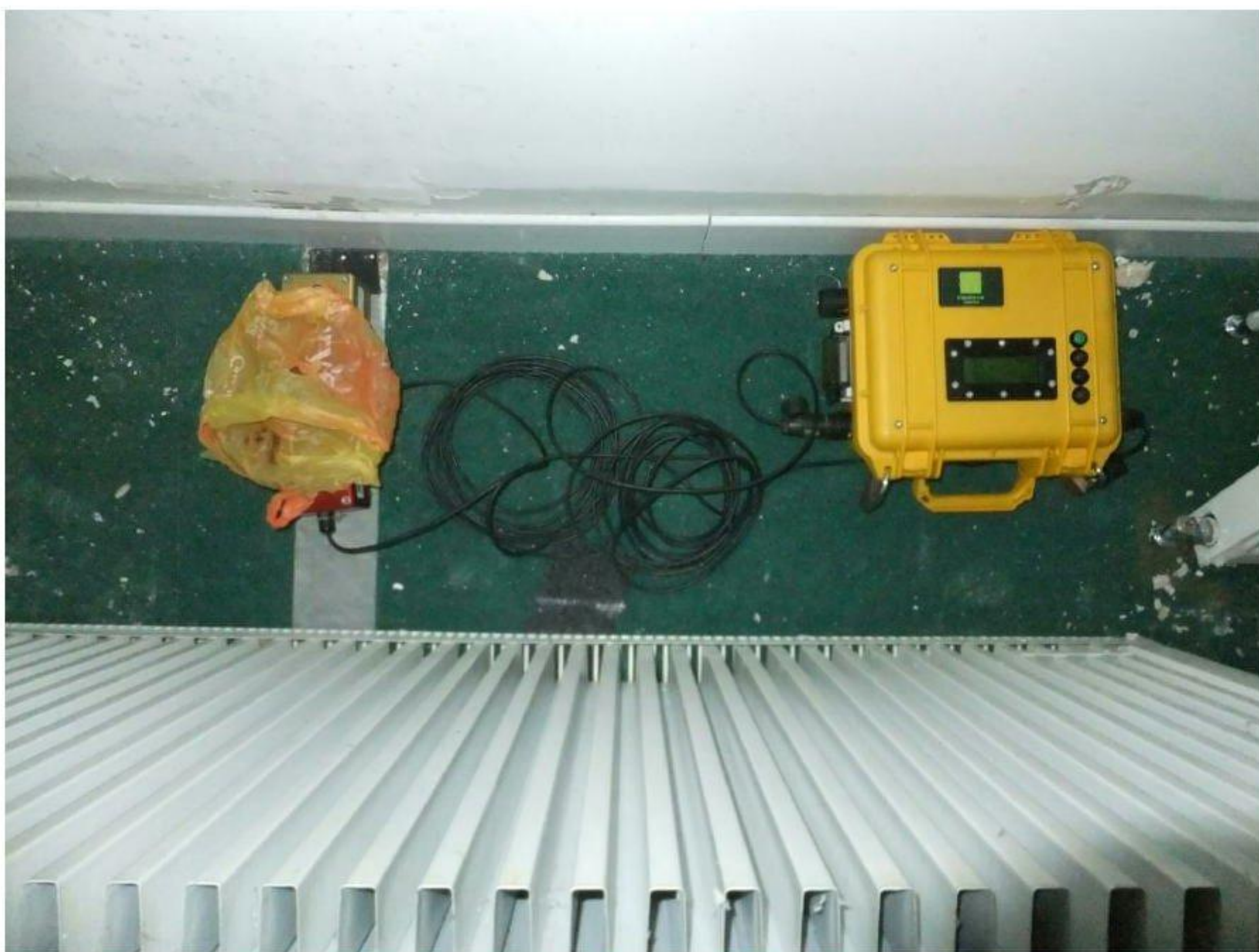
Photo 3 Measurement of groundborne vibration at base of façade towards railway
