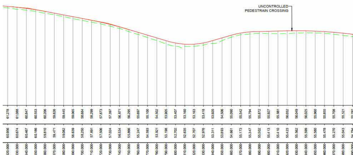
Figure 2-3 – Vertical alignment on crossing approach
