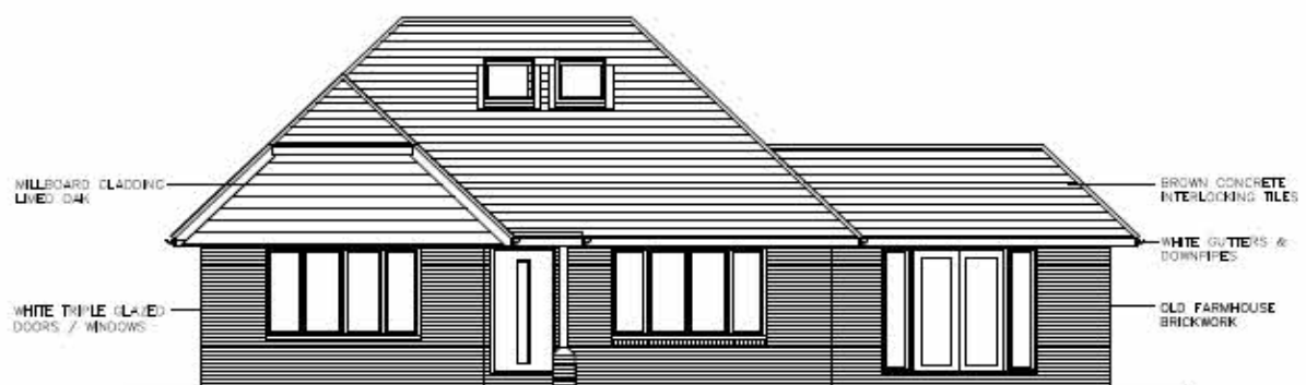
FRONT ELEVATION (SOUTH WEST)
