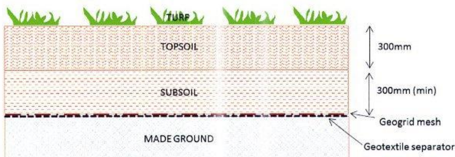
Schematic 1 Topsoil and subsoil cover system where Made Ground is present beneath gardens
