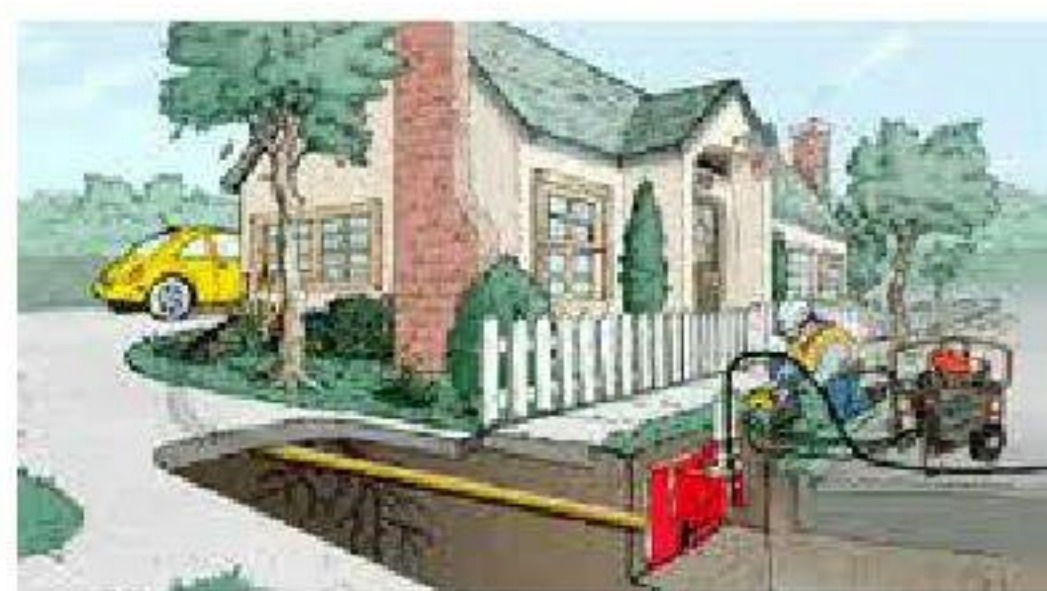
Photo 7: Trenchless insertion of services
