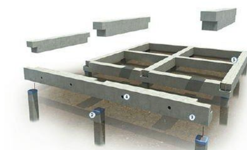
Photo 5: Driven pile foundation with a ventilated air space
