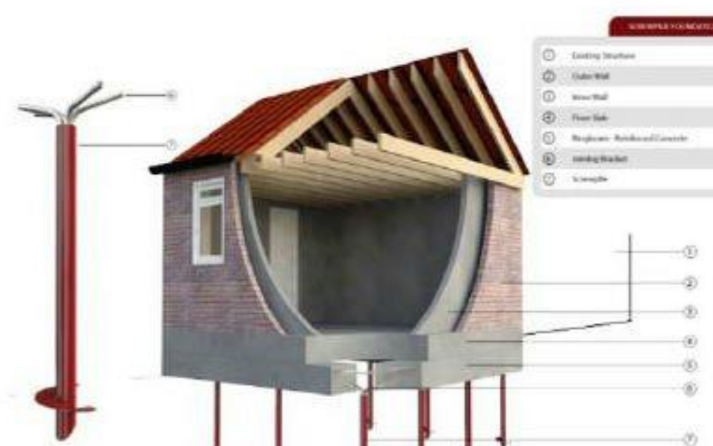
Photo 6: Screw pile foundation with a ventilated air space
