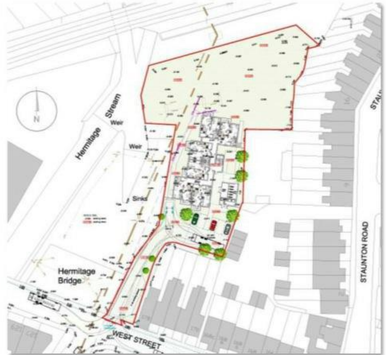
Site layout Plan showing the 600mm sewer (thick brown dashed line)
