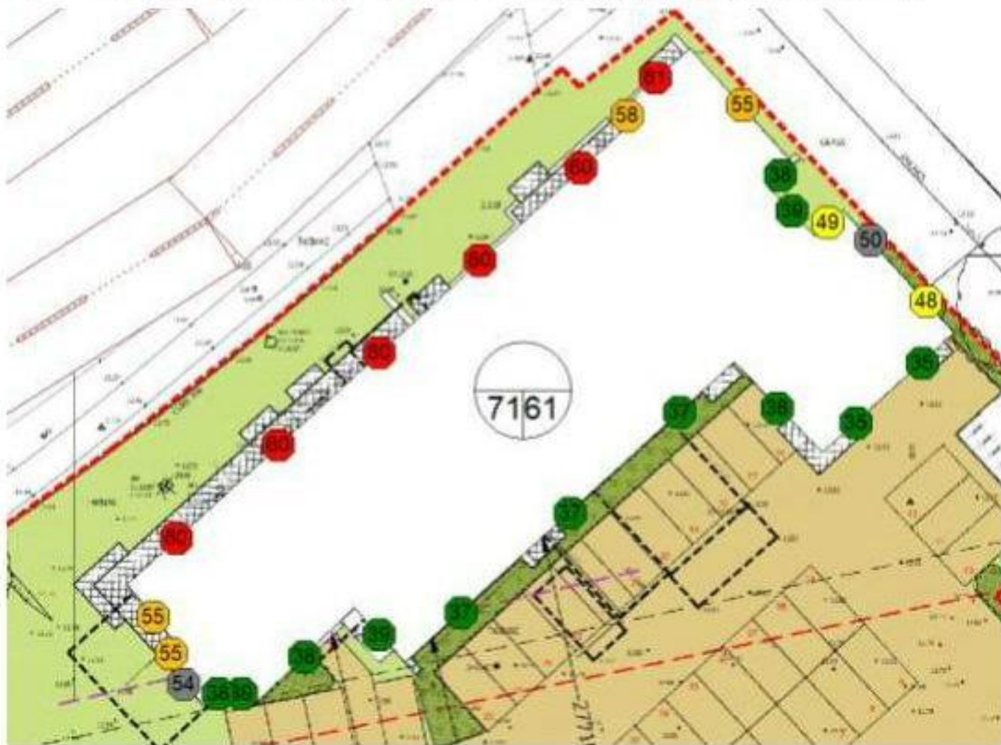
Figure 4: Predicted Night-time Equivalent Noise level L_{Aeq(8 \text{ hours})} at the proposed dwellings
