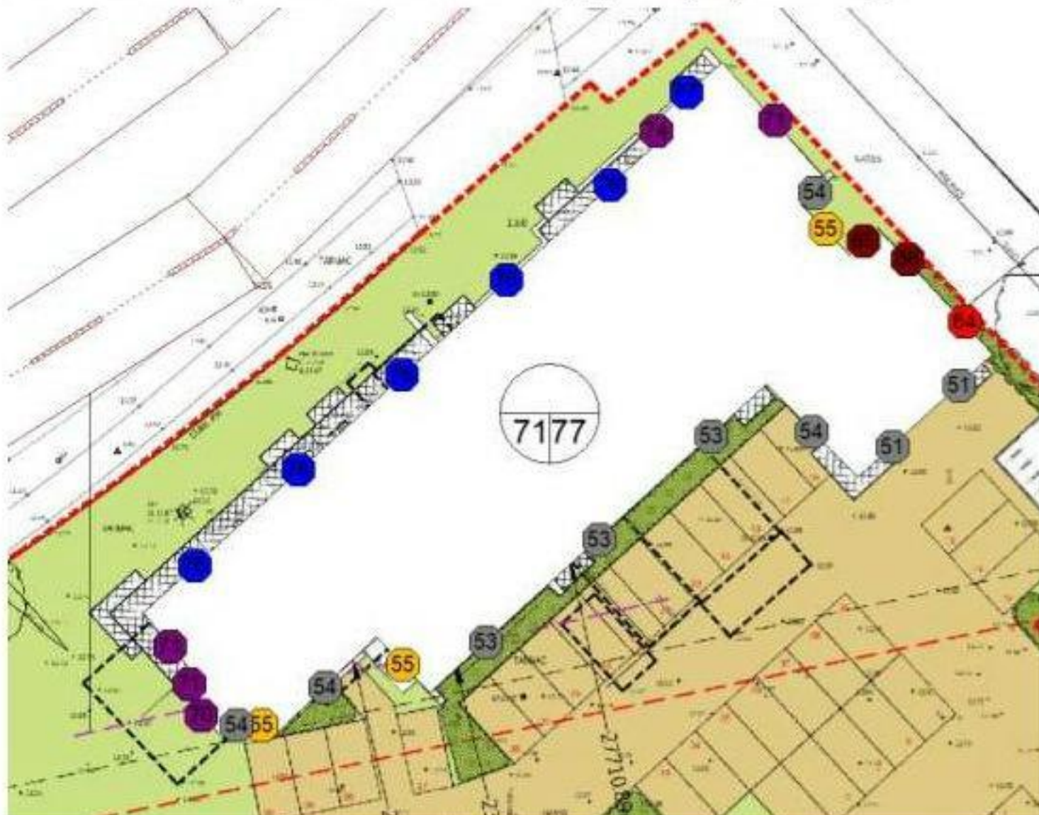
Figure 5: Predicted Night-time Maximum Noise level L_{AFmax} at the proposed dwellings
