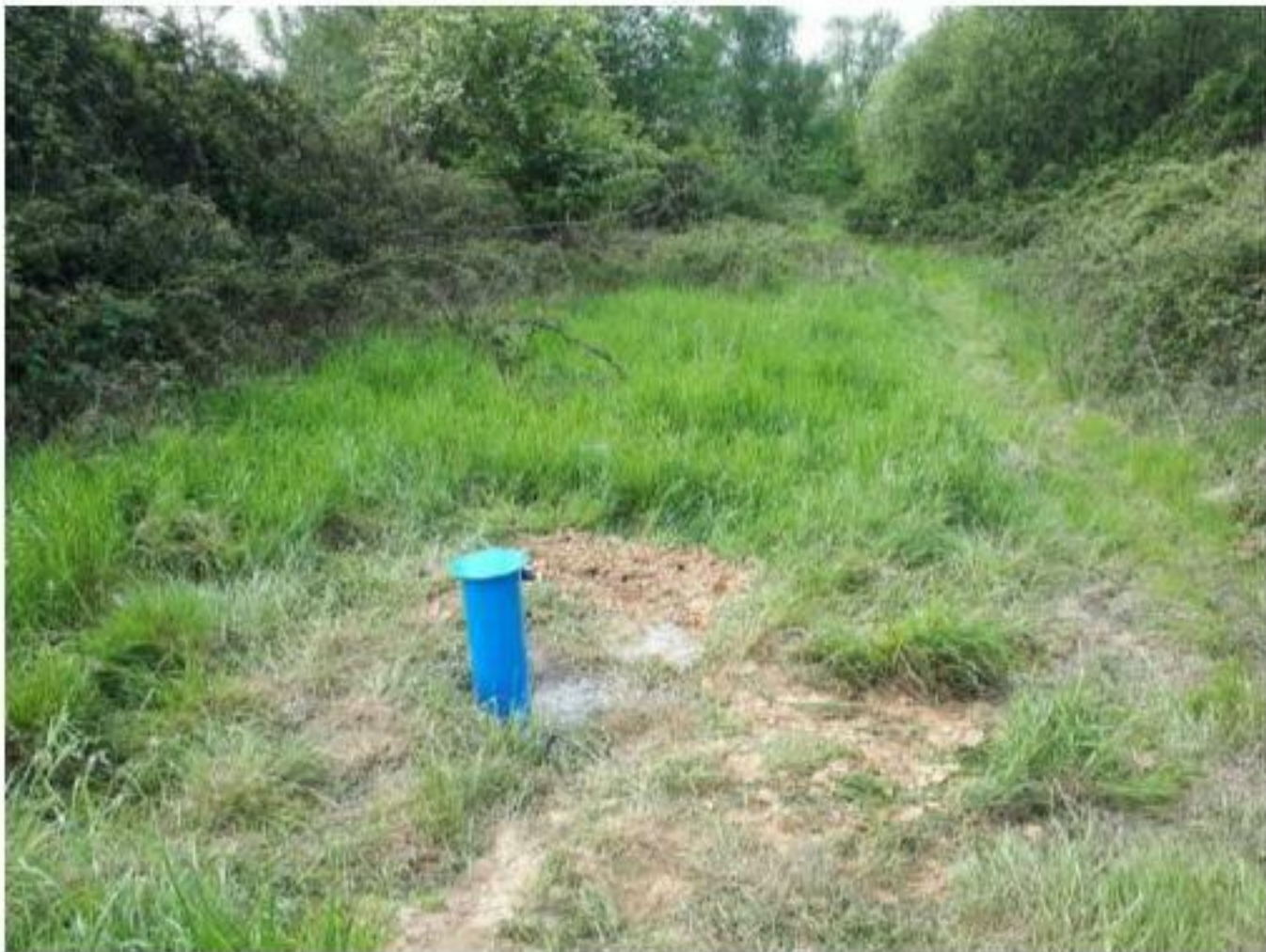
Plate 9: Borehole installation at WS5 with raised cover.
