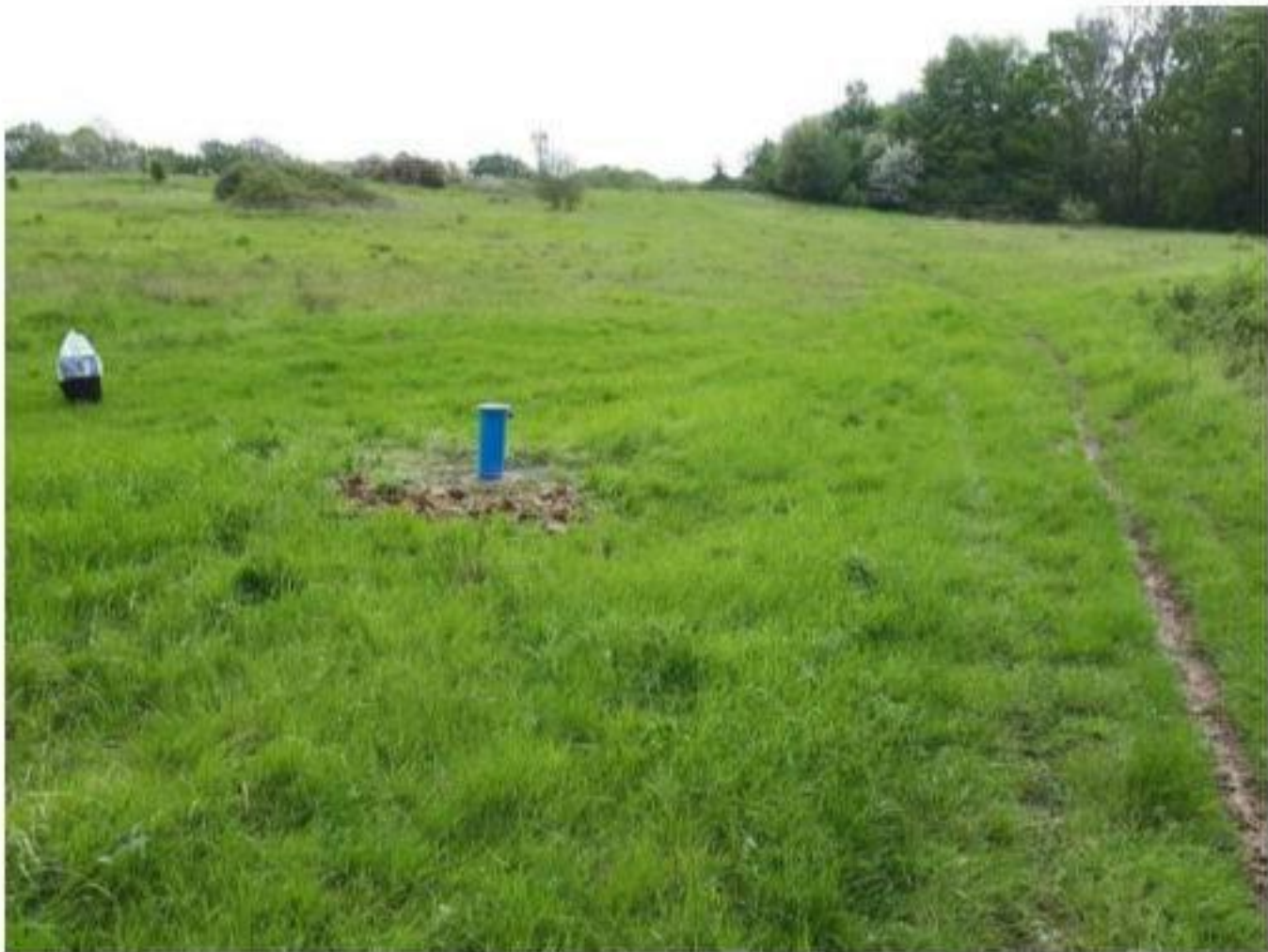
Plate 3: Borehole installation at WS1 with raised cover.
