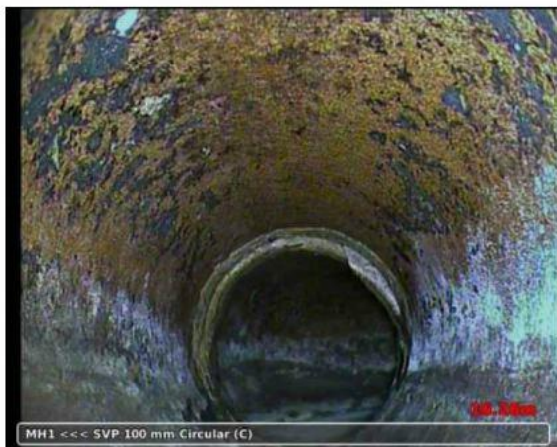
20191010-085806-snap0007.jpg, 00:04:06, 16.26 m Line deviates right
