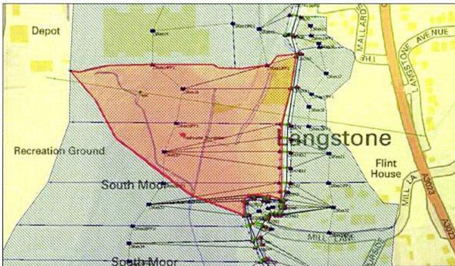
Figure 4.7: InfoWorks Model River Lavant area of available storage capacity
