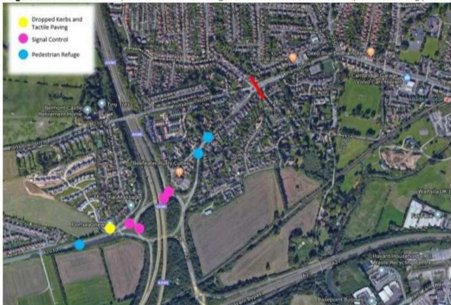
Figure 7: Route north of Rusty Cutter with additional signals and southern side of Bedhampton Hill crossing points
