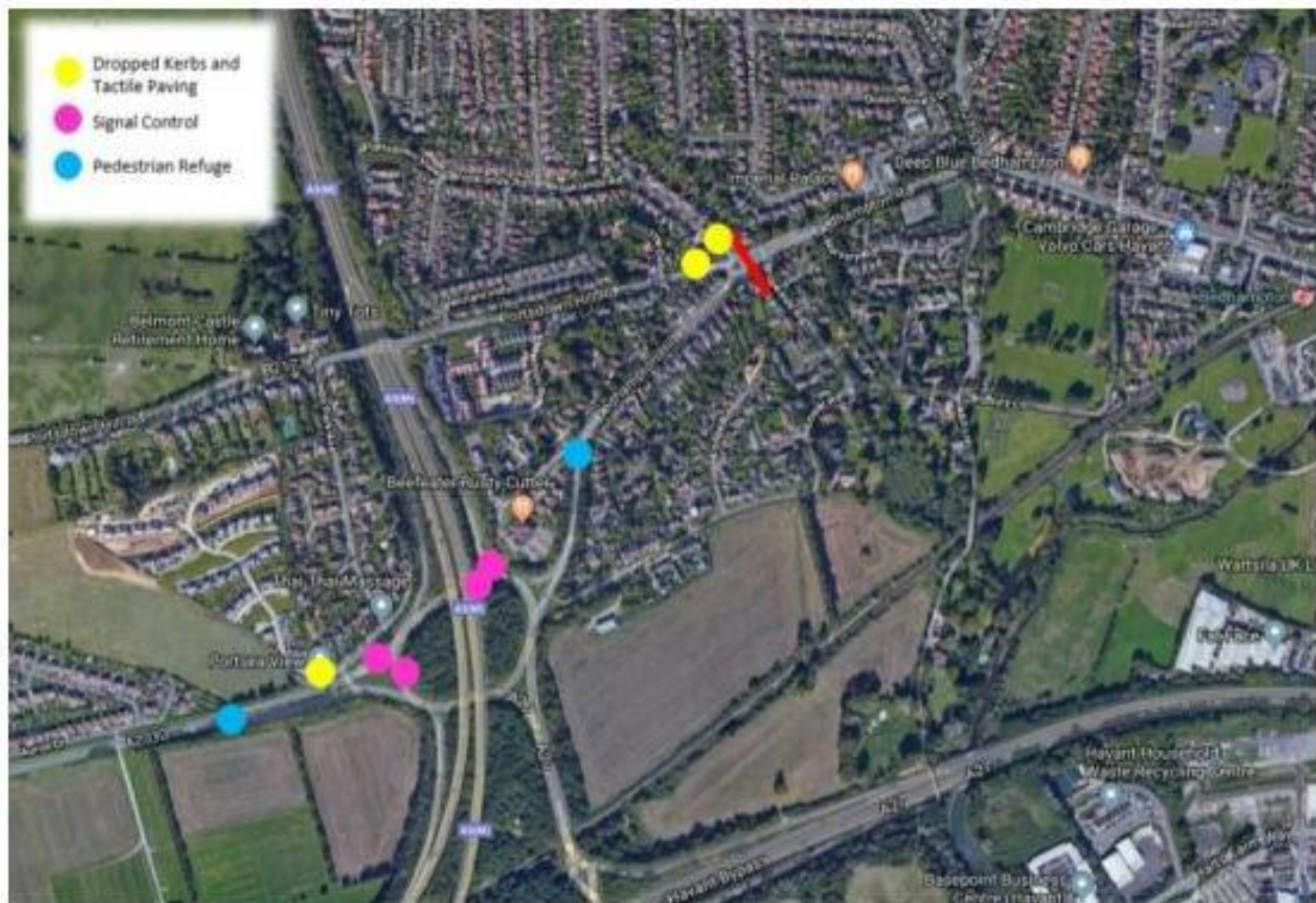
Figure 6: Route north of Rusty Cutter with additional signals and northern side of Bedhampton Hill crossing points
