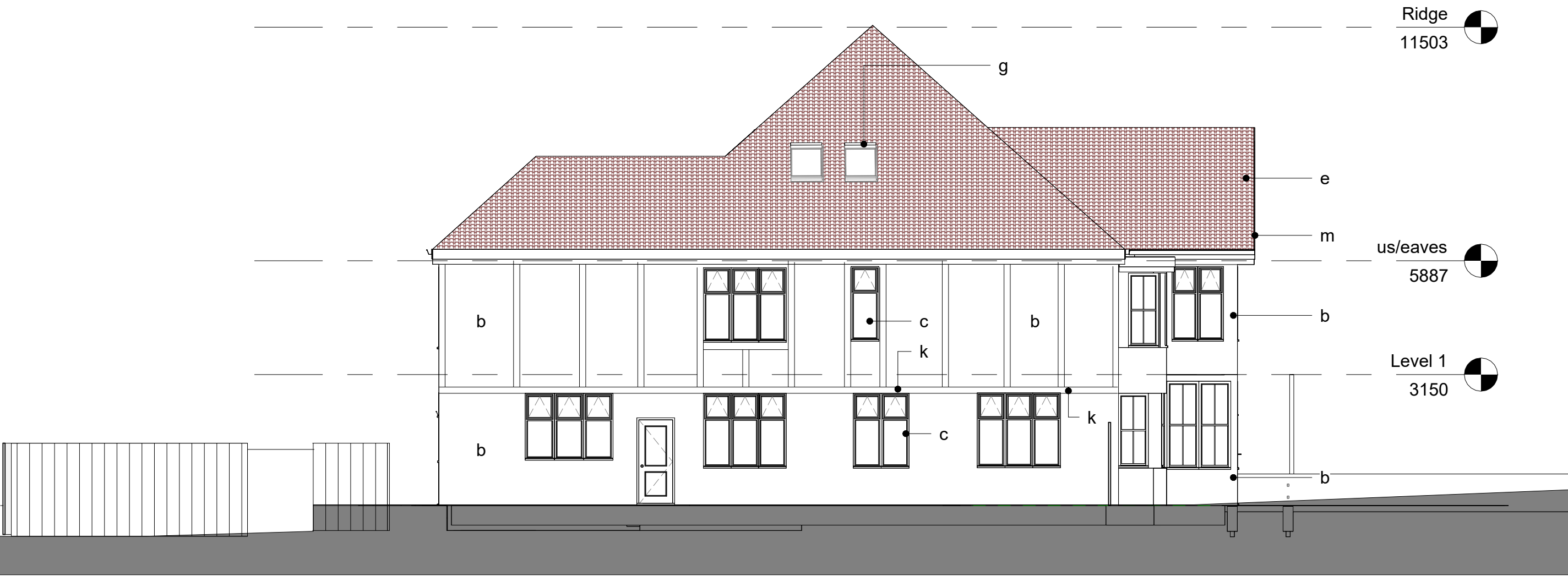
West Elevation as Proposed 1 : 100
