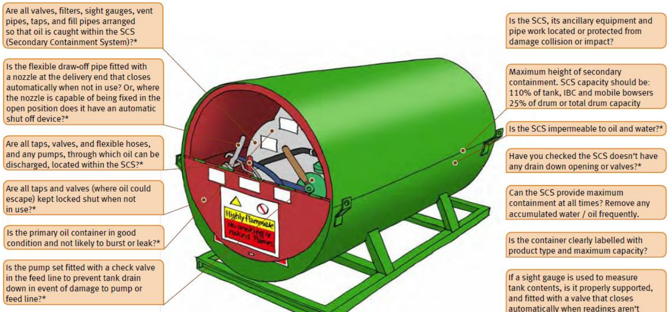
Figure 9 - Illustration of oil storage with a secondary containment system
