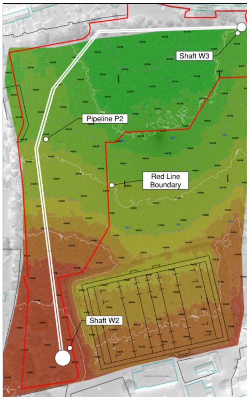
Figure 6.1 Topographical LiDAR Survey (Hooks Lane Playing Fields)
