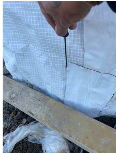
A mechanical point stress test being conducted upon the Corden EPS GRM Self Adhesive Membrane.
