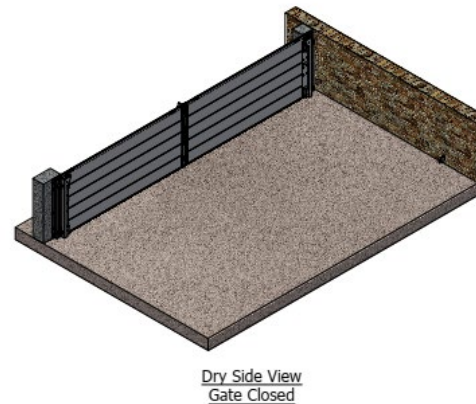
Figure 6.8: High Street Vehicle Flood Gate
