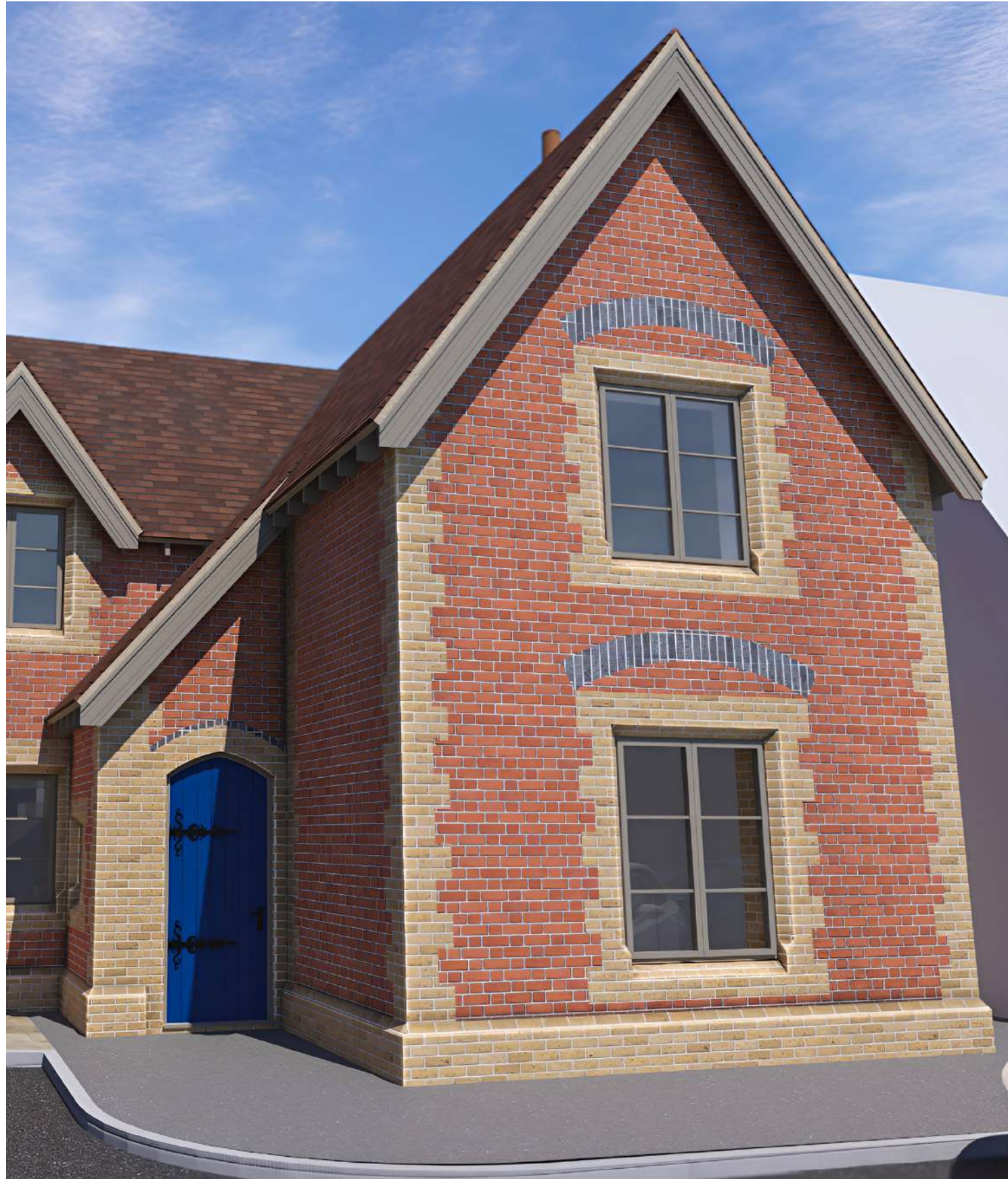
Visual showing improved windows and bargeboards.
