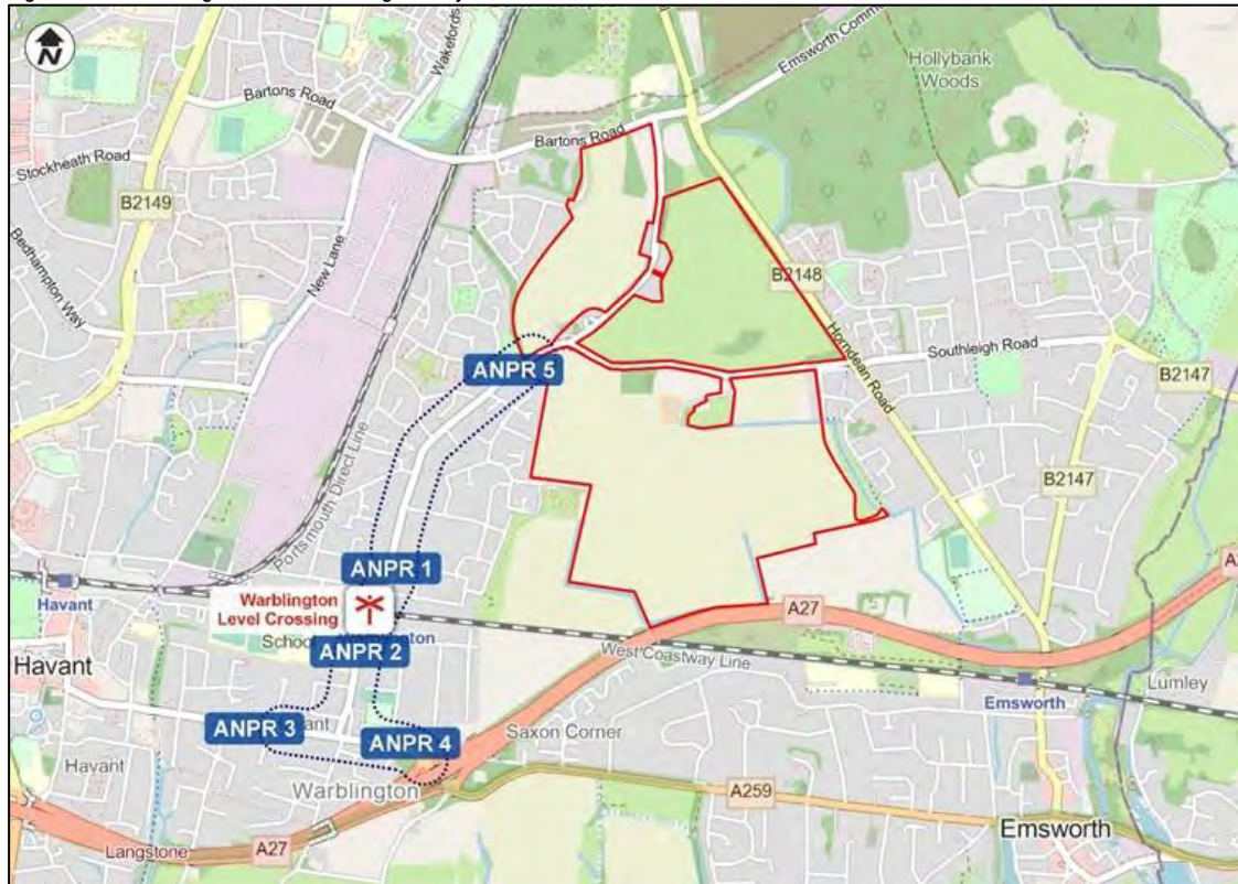
Figure 11.1: Warblington Level Crossing Survey – Location of ANPR Cameras
