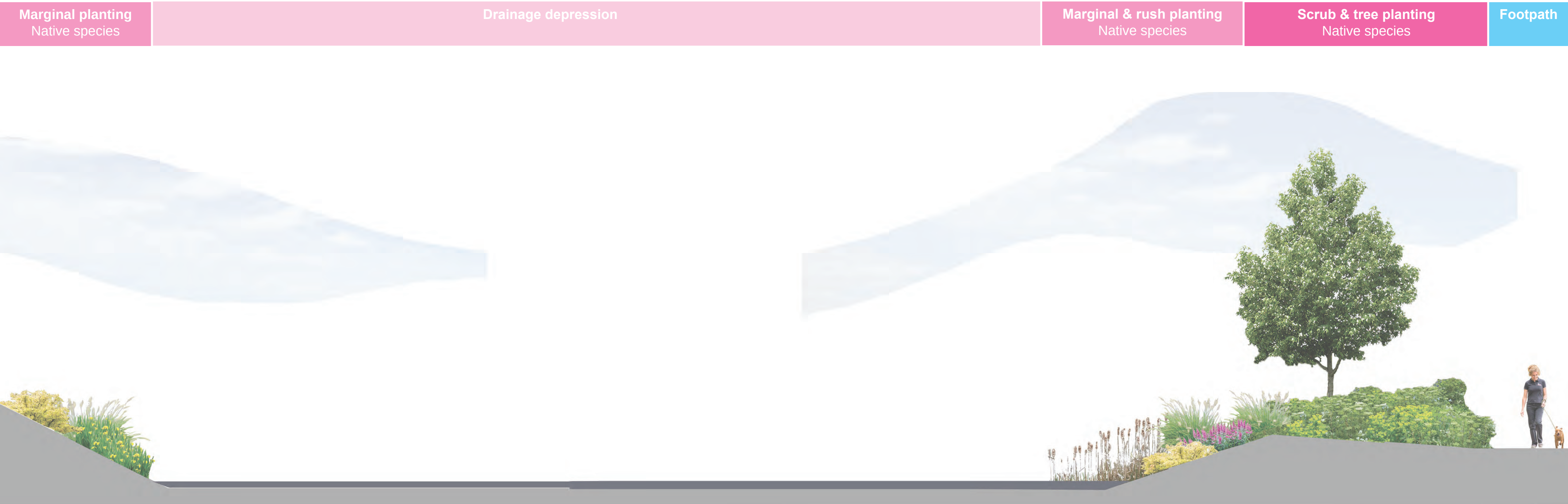
Section through drainage depression space
