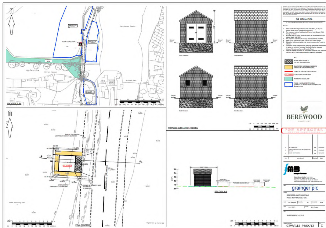
Figure 2.4: Proposed Layout – Phase 4 Substation Works
