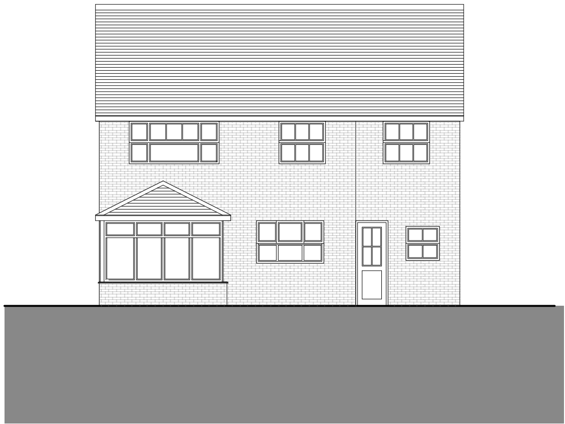
EXISTING REAR ELEVATION 1:100
