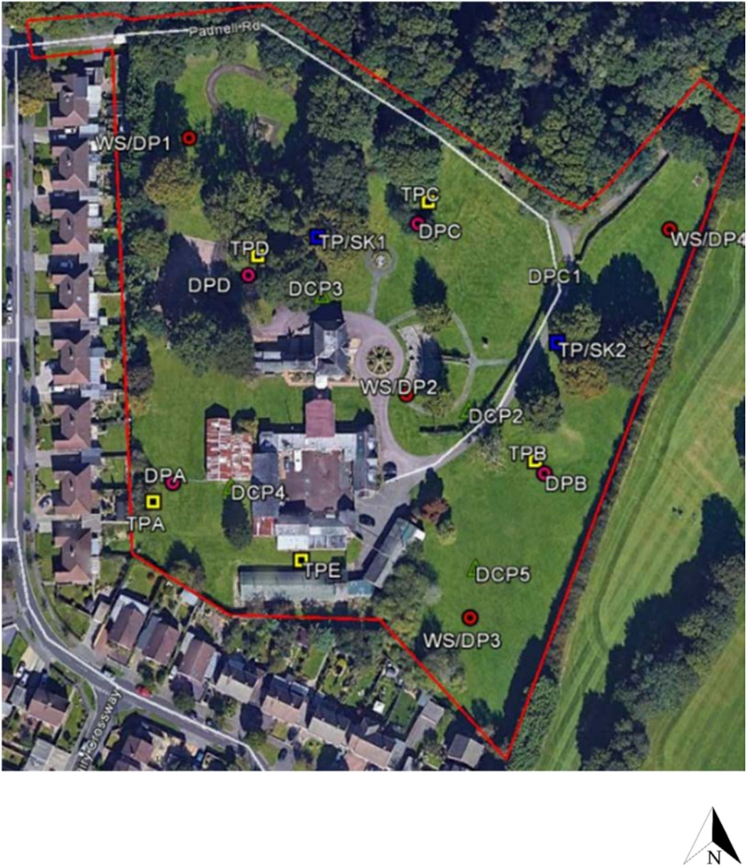
Figure 4 – Exploratory Hole Plan from previous investigation I6362/GIR
