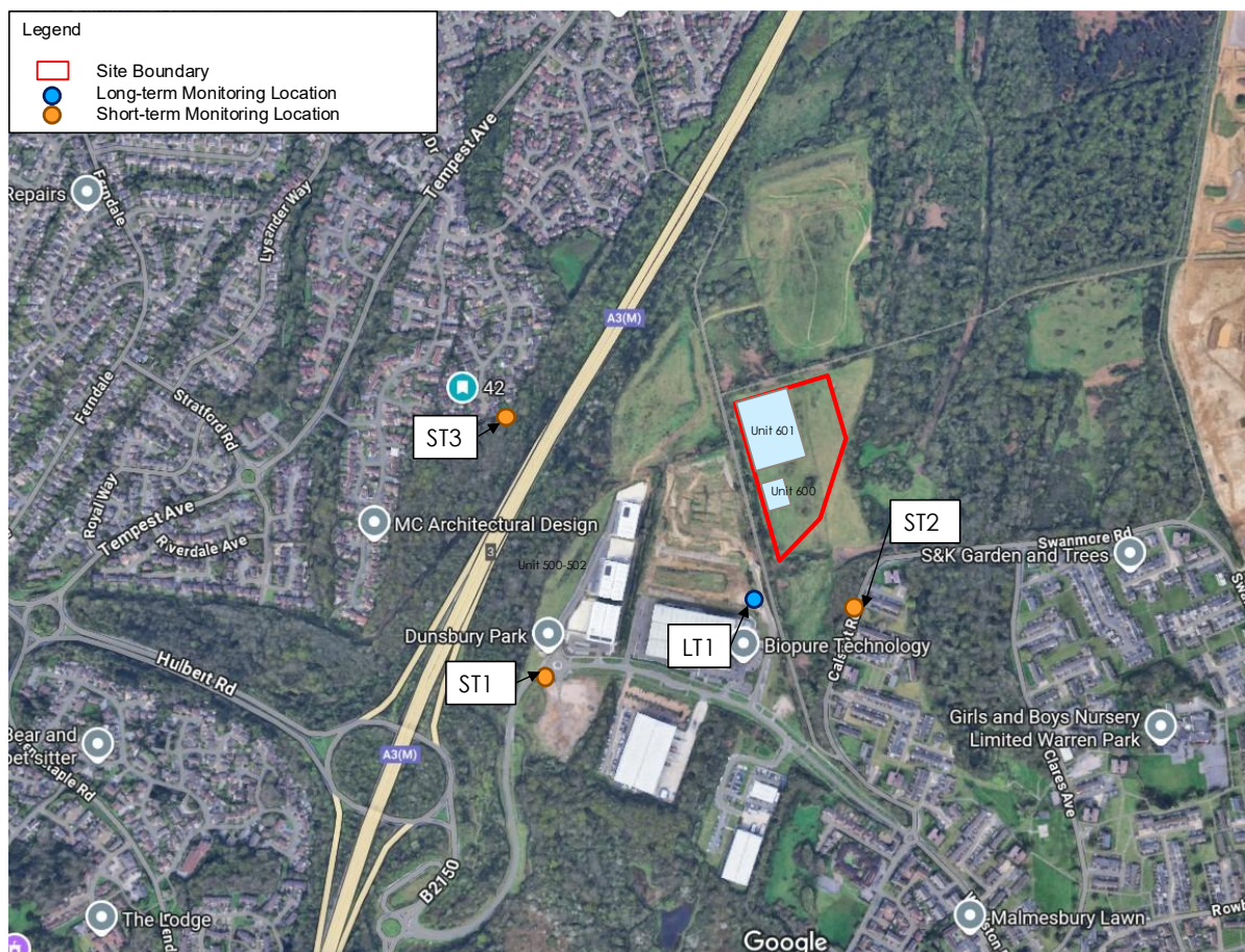
Figure 4 Environmental Noise Survey Locations
