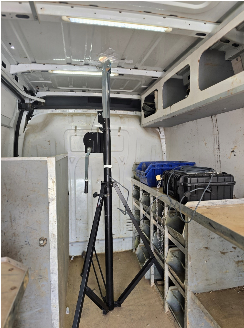
Figure B-1 – Tripod and Sound Level Meter Set Up Within the Van.
