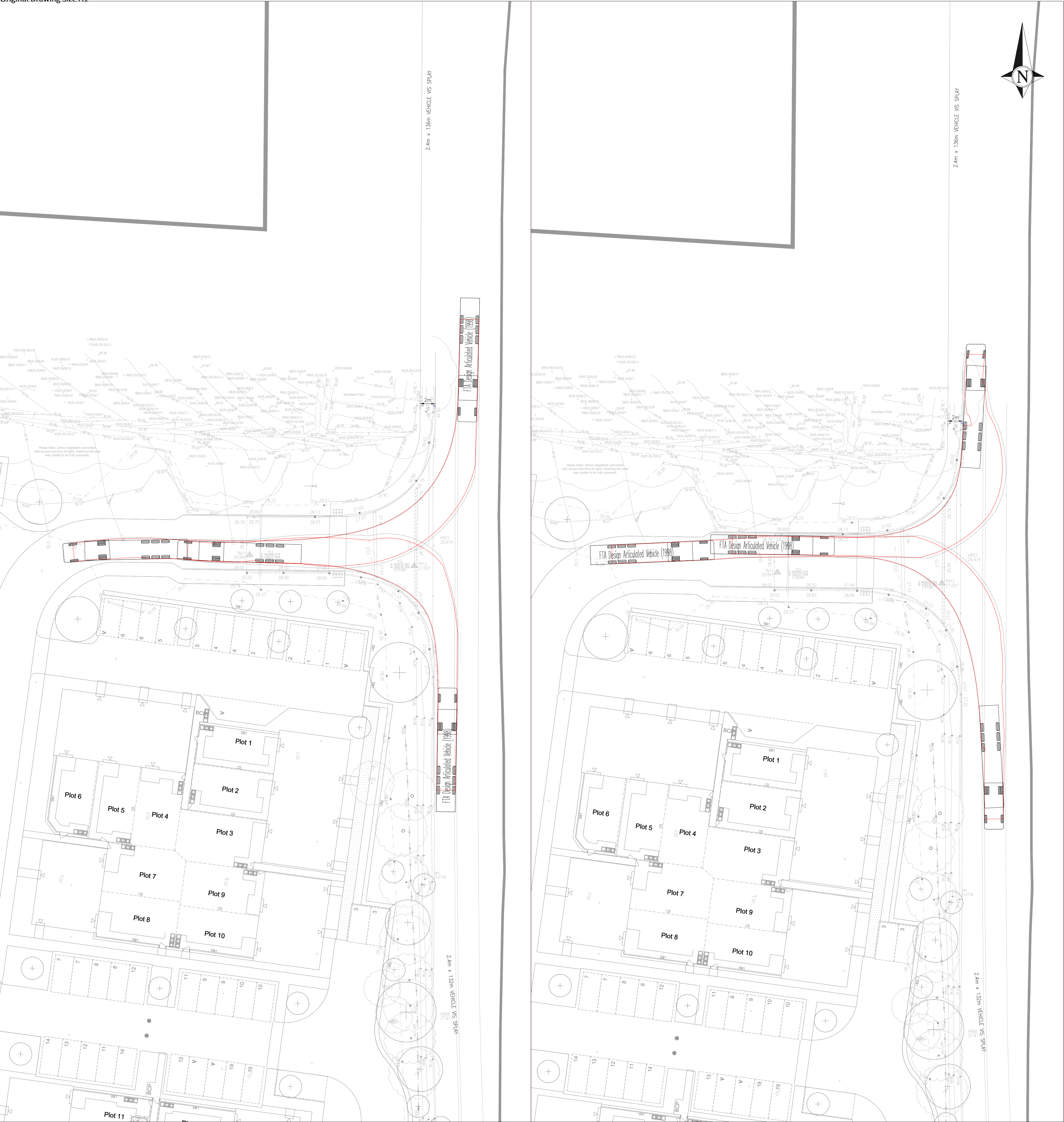
ARTICULATED LORRY INTO THE SITE
