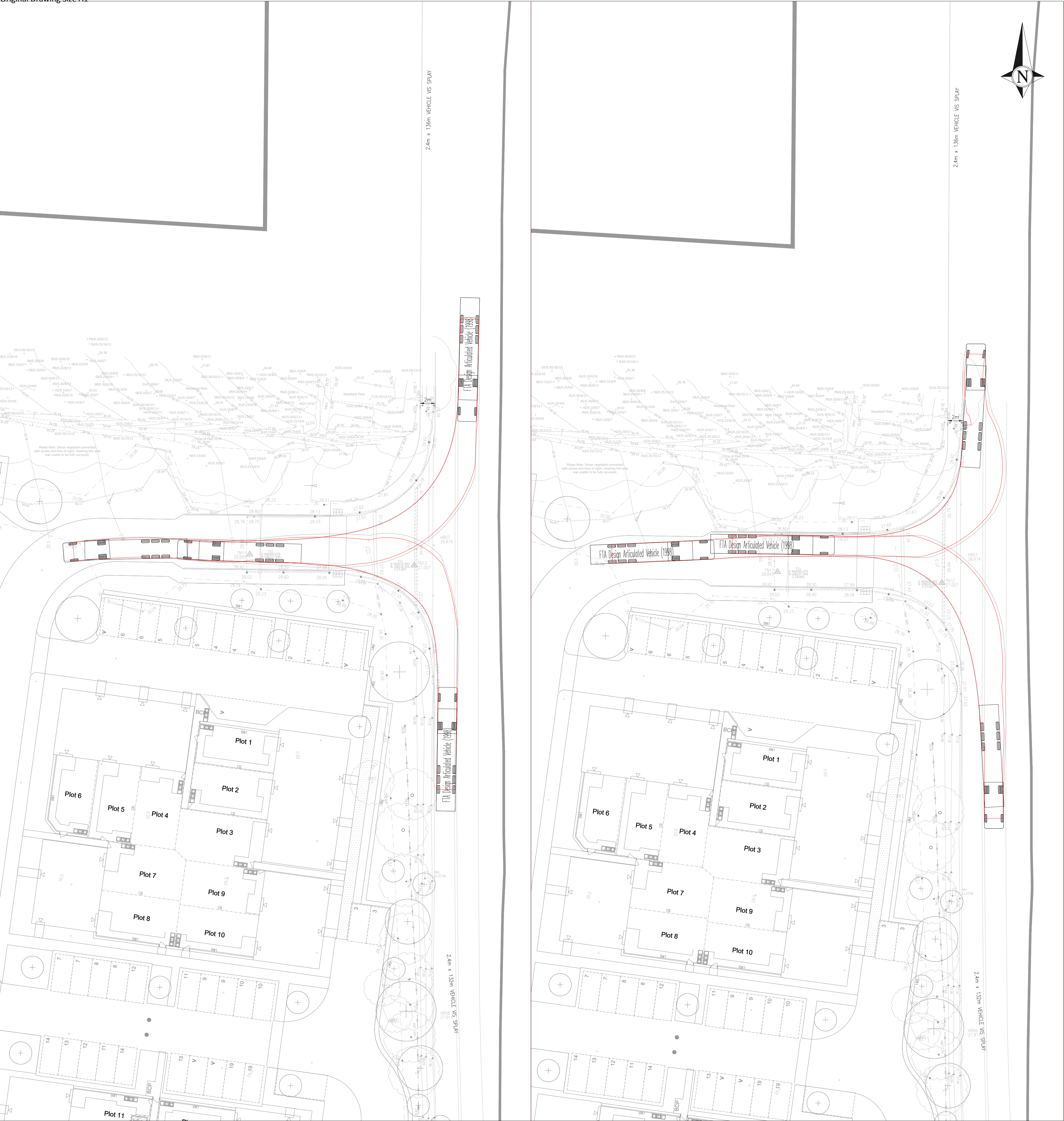
ARTICULATED LORRY INTO THE SITE
